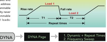
The 63600 also offers a unique dynamic frequency sweep with variable frequencies up to 50kHz. This capability is ideal for determining worst case voltage peaks (see Figure 1). Measurement of the Vpeak (+/-) can be achieved by this function with a sampling rate of 500 kHz (Figure 2). The dynamic loading mode can simulate different loading conditions for most test requirements. Dedicated remote load sensors and control circuits guarantee minimum waveform distortion during dynamic loading.
