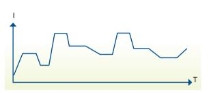
Simulations of all kinds of real current waveforms for battery discharge testing and other applications are possible. (Notebook, Electric car and Electric bike) (Single output channel for UUT)
